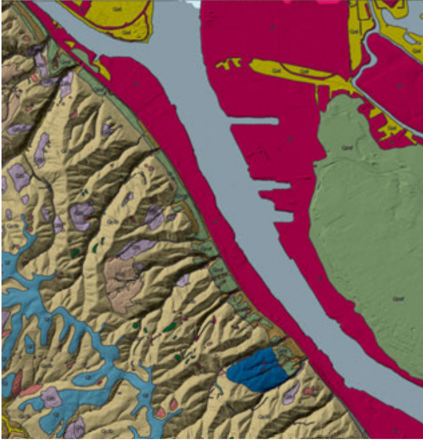
Figure 31: Surface geology map showing areas of fill materials (in pink) adjacent to the river. For geographic reference to Figures 29 and 30, note the three parallel water inlets. (Madin et al, 2008)
